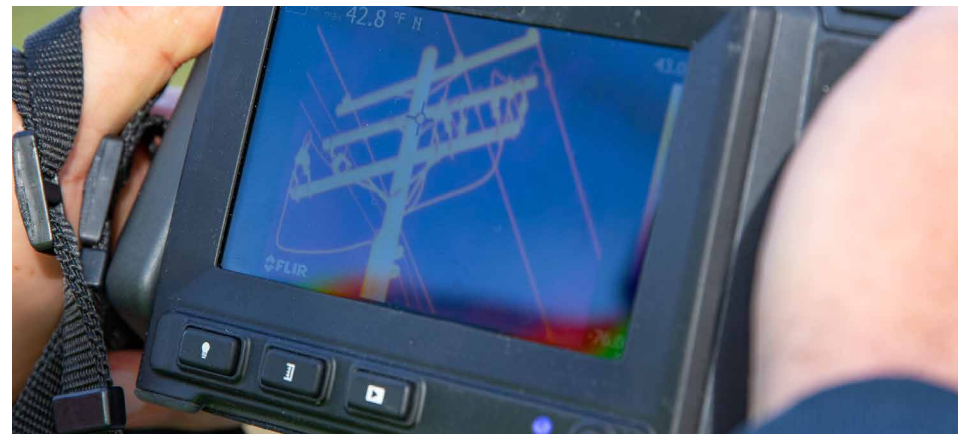
Exelon utilities continue to expand the use of thermal imaging to support employee safety and early detection of potential issues on the system.
