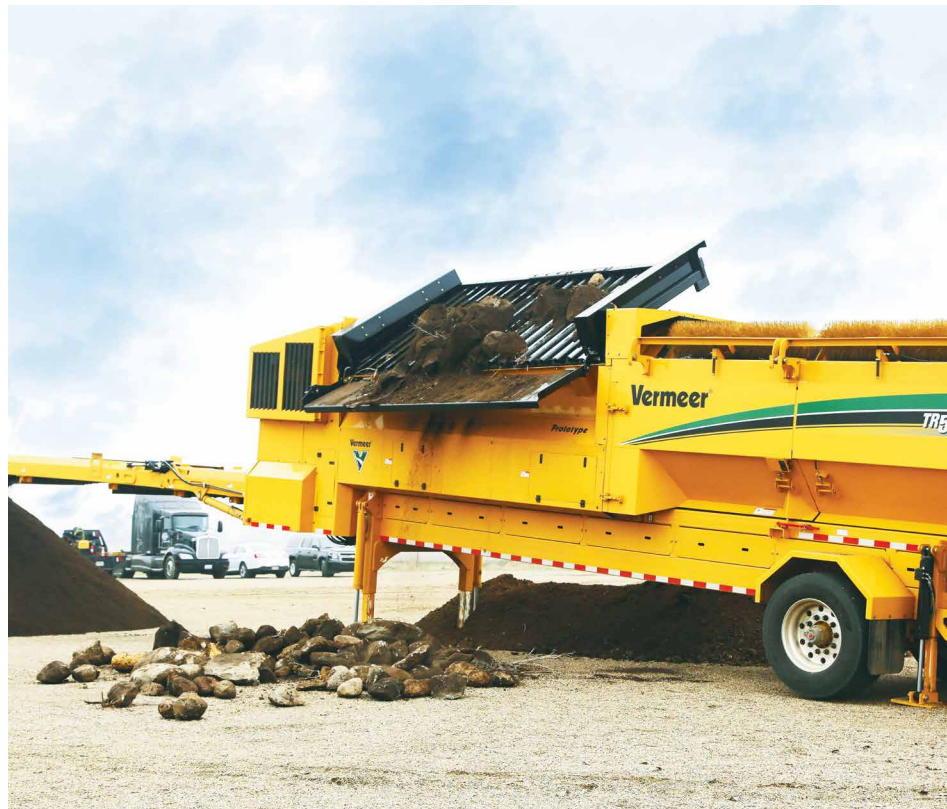
The BGE Gas Division has reduced landfill waste and disposal costs by processing spoil materials for reuse as excavation backfill.
